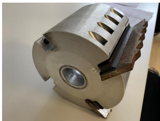
Ice cutter with milling head without safety system with penetrating power
